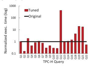
Fig. 1: Non-robust Performance due to Optimization Errors in a State-of-the-art Commercial DBMS when running TPC-H.
