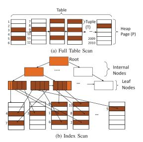
Fig. 2: Access Paths in a DBMS.
