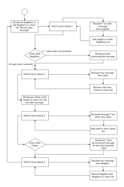
Figure 4.4: Fault-tolerance mechanism in P2P-DIET
