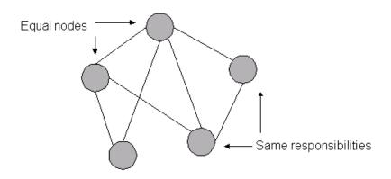
Figure 2.3: Pure peer-to-peer architecture
