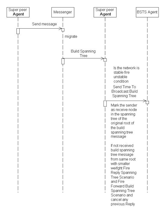
Figure A.32: Forward Build Spanning Tree Scenario
