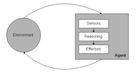
Figure 3.3: A software agent interacts with an environment through sensors and effectors
