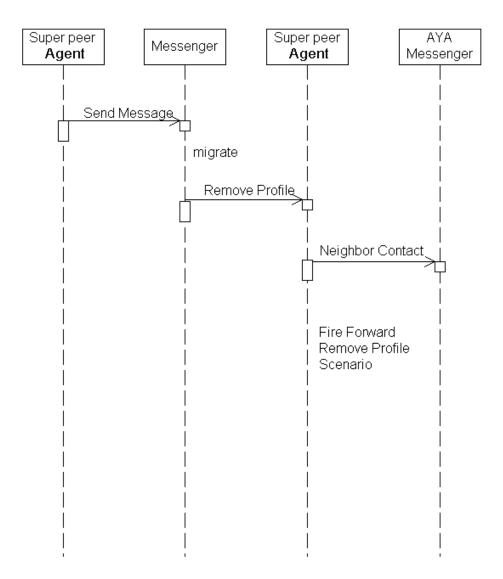
Figure A.9: Forward Remove Profile Scenario
