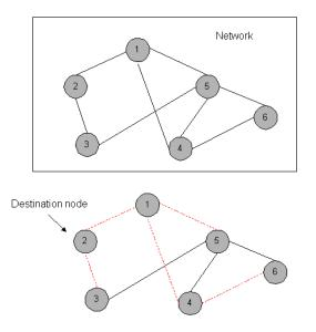
Figure 4.1: An example of a shortest path
