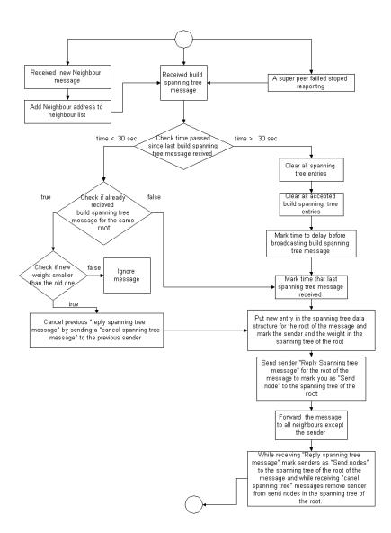
Figure 4.3: A distributed for building spanning trees algorithm.
