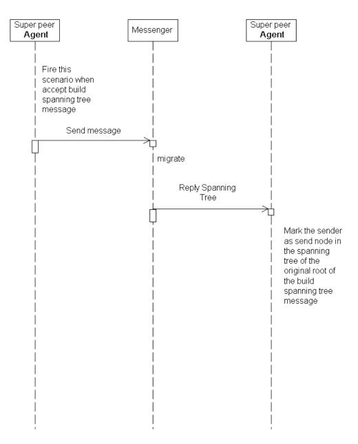
Figure A.33: Reply Spanning Tree Scenario
